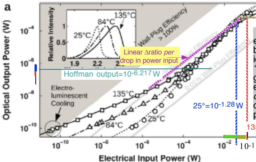
Voltage at which electrical energy falls below light energy is identified on the "power output to input" graph by 135° and 25° electric wattage. Power output to input ratios converge below that point for all temperatures.
