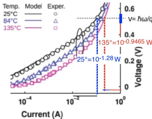
MIT estimated LED voltage at which electrical energy falls below light emission energy
